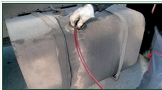
Taking fuel from a tank for laboratory analysis
